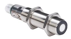
Micro Detectors ultrasonic proximity sensor, tubular, 18mm diameter x 91.6mm body, 316L stainless steel housing, PNP, 4-20 mA analog output, N.O./N.C. selectable output, 150-1600mm sensing distance, 3 Hz switching frequency, IP67, 5-pin M12 quick-disconnect.
