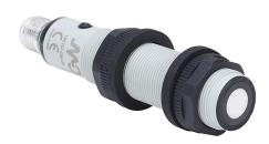
Micro Detectors ultrasonic proximity sensor, tubular, 18mm diameter x 91.6mm body, polybutylene terephthalate housing, PNP, 4-20 mA analog output, N.O./N.C. selectable output, 150-1600mm sensing distance, 3 Hz switching frequency, IP67, 5-pin M12 quick-disconnect.
