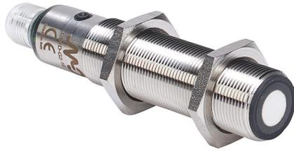
Micro Detectors ultrasonic proximity sensor, tubular, 18mm diameter x 91.6mm body, 316L stainless steel housing, 4-20 mA analog output, 150-1600mm sensing distance, IP67, 4-pin M12 quick-disconnect.
