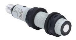
Micro Detectors ultrasonic proximity sensor, tubular, 18mm diameter x 91.6mm body, polybutylene terephthalate housing, 4-20 mA analog output, 150-1600mm sensing distance, IP67, 4-pin M12 quick-disconnect.
