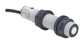
Micro Detectors ultrasonic proximity sensor, tubular, 18mm diameter x 83.6mm body, polybutylene terephthalate housing, 4-20 mA analog output, 150-1600mm sensing distance, IP67, pigtail.
