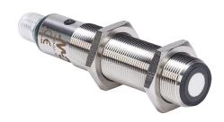
Micro Detectors ultrasonic proximity sensor, tubular, 18mm diameter x 91.6mm body, 316L stainless steel housing, 0-10 VDC analog output, 150-1600mm sensing distance, IP67, 4-pin M12 quick-disconnect.
