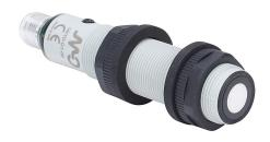
Micro Detectors ultrasonic proximity sensor, tubular, 18mm diameter x 91.6mm body, polybutylene terephthalate housing, 0-10 VDC analog output, 150-1600mm sensing distance, IP67, 4-pin M12 quick-disconnect.
