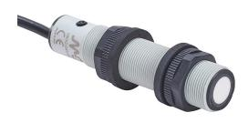
Micro Detectors ultrasonic proximity sensor, tubular, 18mm diameter x 83.6mm body, polybutylene terephthalate housing, PNP, (2) N.O./N.C. selectable outputs, 80-900mm sensing distance, 4 Hz switching frequency, IP67, pigtail.
