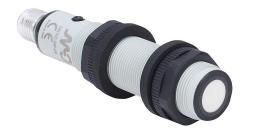
Micro Detectors ultrasonic proximity sensor, tubular, 18mm diameter x 91.6mm body, polybutylene terephthalate housing, PNP, N.O./N.C. selectable output, 80-900mm sensing distance, 4 Hz switching frequency, IP67, 4-pin M12 quick-disconnect.
