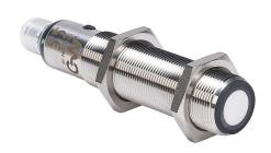
Micro Detectors ultrasonic proximity sensor, tubular, 18mm diameter x 91.6mm body, 316L stainless steel housing, NPN, N.O./ N.C. selectable output, 80-900mm sensing distance, 4 Hz switching frequency, IP67, 4-pin M12 quick-disconnect.
