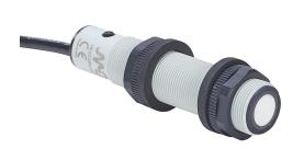
Micro Detectors ultrasonic proximity sensor, tubular, 18mm diameter x 83.6mm body, polybutylene terephthalate housing, NPN, N.O./N.C. selectable output, 80-900mm sensing distance, 4 Hz switching frequency, IP67, pigtail.
