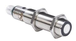
Micro Detectors ultrasonic proximity sensor, tubular, 18mm diameter x 91.6mm body, 316L stainless steel housing, PNP, 0-10 VDC analog output, N.O./N.C. selectable output, 80-900mm sensing distance, 4 Hz switching frequency, IP67, 5-pin M12 quick-disconnect.
