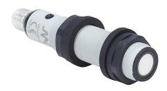
Micro Detectors ultrasonic proximity sensor, tubular, 18mm diameter x 91.6mm body, polybutylene terephthalate housing, PNP, 0-10 VDC analog output, N.O./N.C. selectable output, 80-900mm sensing distance, 4 Hz switching frequency, IP67, 5-pin M12 guick-disconnect.
