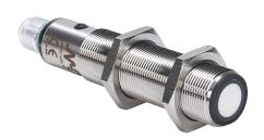
Micro Detectors ultrasonic proximity sensor, tubular, 18mm diameter x 91.6mm body, 316L stainless steel housing, PNP, 4-20 mA analog output, N.O./N.C. selectable output, 80-900mm sensing distance, 4 Hz switching frequency, IP67, 5-pin M12 quick-disconnect.
