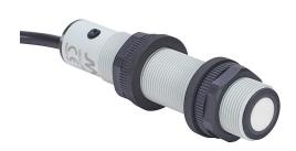
Micro Detectors ultrasonic proximity sensor, tubular, 18mm diameter x 83.6mm body, polybutylene terephthalate housing, PNP, 4-20 mA analog output, N.O./N.C. selectable output, 80-900mm sensing distance, 4 Hz switching frequency, IP67, pigtail.
