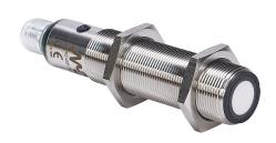
Micro Detectors ultrasonic proximity sensor, tubular, 18mm diameter x 91.6mm body, 316L stainless steel housing, 4-20 mA analog output, 80-900mm sensing distance, IP67, 4-pin M12 quick-disconnect.
