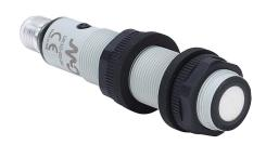
Micro Detectors ultrasonic proximity sensor, tubular, 18mm diameter x 91.6mm body, polybutylene terephthalate housing, 4-20 mA analog output, 80-900mm sensing distance, IP67, 4-pin M12 quick-disconnect.
