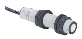
Micro Detectors ultrasonic proximity sensor, tubular, 18mm diameter x 83.6mm body, polybutylene terephthalate housing, 4-20 mA analog output, 80-900mm sensing distance, IP67, pigtail.
