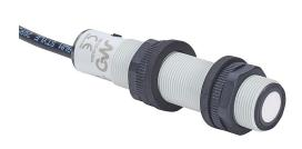
Micro Detectors ultrasonic proximity sensor, tubular, 18mm diameter x 83.6mm body, polybutylene terephthalate housing, 4-20 mA analog output, 80-900mm sensing distance, IP67, pigtail.
