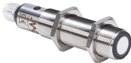
Micro Detectors ultrasonic proximity sensor, tubular, 18mm diameter x 91.6mm body, 316L stainless steel housing, 0-10 VDC analog output, 80-900mm sensing distance, IP67, 4-pin M12 quick-disconnect.
