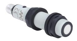
Micro Detectors ultrasonic proximity sensor, tubular, 18mm diameter x 91.6mm body, polybutylene terephthalate housing, 0-10 VDC analog output, 80-900mm sensing distance, IP67, 4-pin M12 quick-disconnect.
