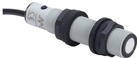
Micro Detectors ultrasonic proximity sensor, tubular, 18mm diameter x 83.6mm body, polybutylene terephthalate housing, 0-10 VDC analog output, 80-900mm sensing distance, IP67, pigtail.
