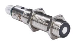
Micro Detectors ultrasonic proximity sensor, tubular, 18mm diameter x 91.6mm body, 316L stainless steel housing, PNP, (2) N.O./N.C. selectable outputs, 50-400mm sensing distance, 10 Hz switching frequency, IP67, 5-pin M12 quick-disconnect.
