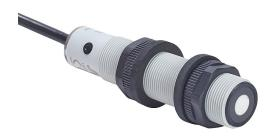
Micro Detectors ultrasonic proximity sensor, tubular, 18mm diameter x 83.6mm body, polybutylene terephthalate housing, PNP, (2) N.O./N.C. selectable outputs, 50-400mm sensing distance, 10 Hz switching frequency, IP67, pigtail.
