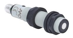
Micro Detectors ultrasonic proximity sensor, tubular, 18mm diameter x 91.6mm body, polybutylene terephthalate housing, PNP, N.O./N.C. selectable output, 50-400mm sensing distance, 10 Hz switching frequency, IP67, 4-pin M12 quick-disconnect.
