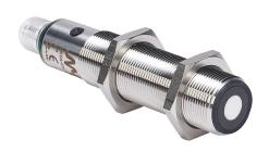
Micro Detectors ultrasonic proximity sensor, tubular, 18mm diameter x 91.6mm body, 316L stainless steel housing, NPN, N.O./ N.C. selectable output, 50-400mm sensing distance, 10 Hz switching frequency, IP67, 4-pin M12 quick-disconnect.
