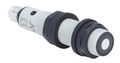
Micro Detectors ultrasonic proximity sensor, tubular, 18mm diameter x 91.6mm body, polybutylene terephthalate housing, NPN, N.O./N.C. selectable output, 50-400mm sensing distance, 10 Hz switching frequency, IP67, 4-pin M12 quick-disconnect.
