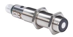
Micro Detectors ultrasonic proximity sensor, tubular, 18mm diameter x 91.6mm body, 316L stainless steel housing, PNP, 0-10 VDC analog output, N.O./N.C. selectable output, 50-400mm sensing distance, 10 Hz switching frequency, IP67, 5-pin M12 quick-disconnect.
