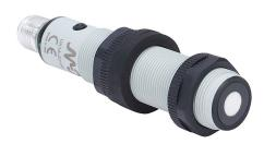
Micro Detectors ultrasonic proximity sensor, tubular, 18mm diameter x 91.6mm body, polybutylene terephthalate housing, PNP, 0-10 VDC analog output, N.O./N.C. selectable output, 50-400mm sensing distance, 10 Hz switching frequency, IP67, 5-pin M12 guick-disconnect.
