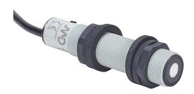
Micro Detectors ultrasonic proximity sensor, tubular, 18mm diameter x 83.6mm body, polybutylene terephthalate housing, PNP, 0-10 VDC analog output, N.O./N.C. selectable output, 50-400mm sensing distance, 10 Hz switching frequency, IP67, pigtail.
