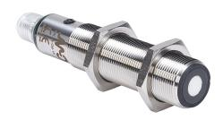
Micro Detectors ultrasonic proximity sensor, tubular, 18mm diameter x 91.6mm body, 316L stainless steel housing, PNP, 4-20 mA analog output, N.O./N.C. selectable output, 50-400mm sensing distance, 10 Hz switching frequency, IP67, 5-pin M12 quick-disconnect.
