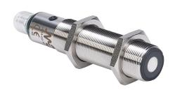
Micro Detectors ultrasonic proximity sensor, tubular, 18mm diameter x 91.6mm body, 316L stainless steel housing, 4-20 mA analog output, 50-400mm sensing distance, IP67, 4-pin M12 quick-disconnect.
