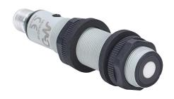
Micro Detectors ultrasonic proximity sensor, tubular, 18mm diameter x 91.6mm body, polybutylene terephthalate housing, 4-20 mA analog output, 50-400mm sensing distance, IP67, 4-pin M12 quick-disconnect.
