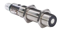
Micro Detectors ultrasonic proximity sensor, tubular, 18mm diameter x 91.6mm body, 316L stainless steel housing, 0-10 VDC analog output, 50-400mm sensing distance, IP67, 4-pin M12 quick-disconnect.
