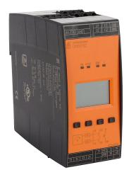
Dold safety relay, speed monitoring, multi delay functions, (2) NPN sensor inputs, 2-channel, 24 VDC, (2) N.O. safety output(s), (2) N.O. monitoring output(s), pluggable screw terminals.
