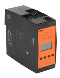
Dold safety relay, motor standstill, speed and safety gate monitoring, multi delay functions, (2) PNP or NPN sensor inputs and/or (1) encoder, 2-channel, 24 VDC, (4) N.O. safety output(s), (2) status monitoring output(s), pluggable screw terminals.
