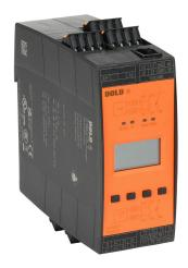
Dold safety relay, motor standstill, speed and safety gate monitoring, multi delay functions, (2) PNP or NPN sensor inputs and/or (1) encoder, 2-channel, 24 VDC, (4) N.O. safety output(s), (2) status monitoring output(s), push-in cage clamp.
