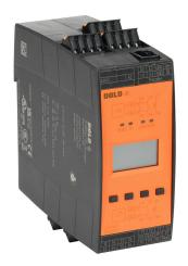
Dold safety relay, motor standstill, speed and safety gate monitoring, multi delay functions, (2) PNP or NPN sensor inputs and/or (1) encoder, 2-channel, 110-240 VAC/VDC, (4) N.O. safety output(s), (2) status monitoring output(s), push-in cage clamp.
