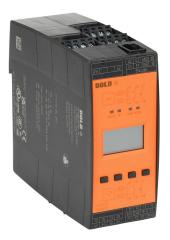
Dold safety relay, motor standstill, speed and safety gate monitoring, multi delay functions, (2) NAMUR sensor inputs and/ or (1) encoder, 2-channel, 24 VDC, (4) N.O. safety output(s), (2) status monitoring output(s), pluggable screw terminals.
