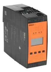
Dold safety relay, motor standstill, speed and safety gate monitoring, multi delay functions, (2) NAMUR sensor inputs and/ or (1) encoder, 2-channel, 110-240 VAC/VDC, (4) N.O. safety output(s), (2) status monitoring output(s), pluggable screw terminals.
