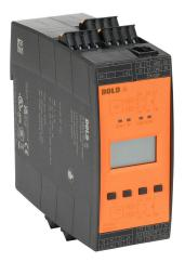
Dold safety relay, motor standstill, speed and safety gate monitoring, multi delay functions, (2) NAMUR sensor inputs and/ or (1) encoder, 2-channel, 24 VDC, (4) N.O. safety output(s), (2) status monitoring output(s), push-in cage clamp.
