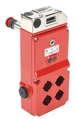
IDEM UGB universal gate box, tongue (key) interlock uniquely coded RFID, rear release with rear release, solenoid, 24 VDC to unlock, 3000N holding force, 4 station, (2) N.C. safety output(s), (2) status monitoring output(s), die-cast aluminum body.
