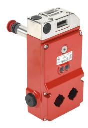
IDEM UGB universal gate box, tongue (key) interlock uniquely coded RFID, rear release with rear release, solenoid, 24 VDC to unlock, 3000N holding force, 2 station, (2) N.C. safety output(s), (2) status monitoring output(s), die-cast aluminum body.
