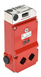
IDEM UGB universal gate box, tongue (key) interlock uniquely coded RFID, solenoid, 24 VDC to unlock, 3000N holding force, 2 station, (2) N.C. safety output(s), (2) status monitoring output(s), die-cast aluminum body, (3) M20 cable entry.
