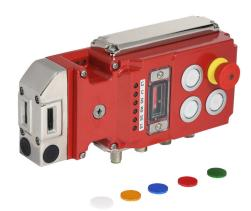
IDEM UGB-NET networked gate box, CIP-Safety, tongue (key) interlock uniquely coded RFID, 4 station, left hand, solenoid, 24 VDC to unlock, die-cast aluminum body.
