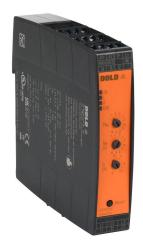
Dold MINISTART 9256 series smart compact motor starter, 9A, 200–480 VAC at 3-phase, Class 5/10A, rated for 30 start/hour, internally bypassed, 22 mm frame. With soft start function.
