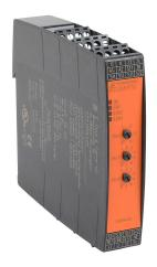
Dold safety relay, (2) independent multi-function, 2-channel, 24 VDC, (4) N.O. safety output(s), (2) N.O. monitoring output(s), pluggable screw terminals.
