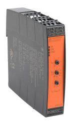
Dold safety relay, emergency stop, multi delay functions, 0.1 to 300 seconds, 2-channel, 24 VDC, (2) N.O. time delay safety output(s), (1) N.O. time delay monitoring output(s), pluggable screw terminals.
