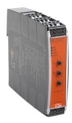
Dold safety relay, light curtain controller, multi delay functions, 0.1 to 300 seconds, 2-channel, 24 VDC, (2) N.O. and (2) N.O. time delay safety output(s), (1) N.O. and (1) N.O. time delay monitoring output(s), pluggable screw terminals.
