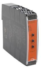
Dold safety relay, emergency stop, multi delay functions, 0.1 to 300 seconds, 2-channel, 24 VDC, (2) N.O. and (2) N.O. time delay safety output(s), (1) N.O. and (1) N.O. time delay monitoring output(s), pluggable screw terminals.
