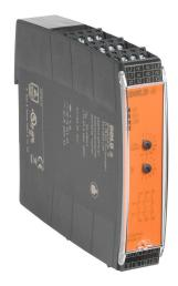
Dold safety relay, motor standstill monitoring, 20-400 mV, 2-channel, 24 VDC, (2) N.O. and (1) N.C. safety output(s), pluggable screw terminals.
